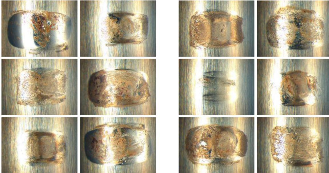
The bearings are 1.3 hours pre-damaged with very small swivel angles of  $\pm 0.5^\circ$  and a force of 3 kN
